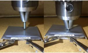
Results here also closely resembled short circuit results (since the nail internally shorts the cell). Cells leaked less than a tenth of a milliliter of electrolyte.
