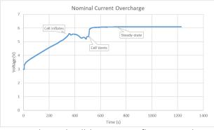
An overcharged cell begins to inflate around 5.8V, losing some voltage until it vents between the tabs.
