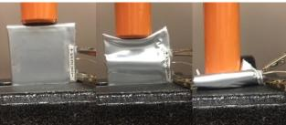
Crushed cells worked normally until crushed fully (right of image) to the point of slicing open the cell enclosure on the vice grips, releasing less than a tenth of a milliliter of electrolyte.
